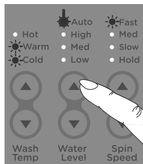
Fig.14 Selecting AUTO water level
